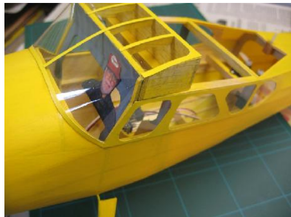
Cessna 195 showing cut windscreen frame strips.
